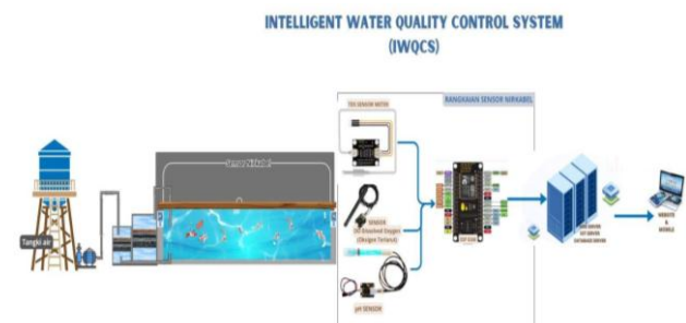
Gambar 4. Skema Teknologi Intelligent Water Quality Control System
